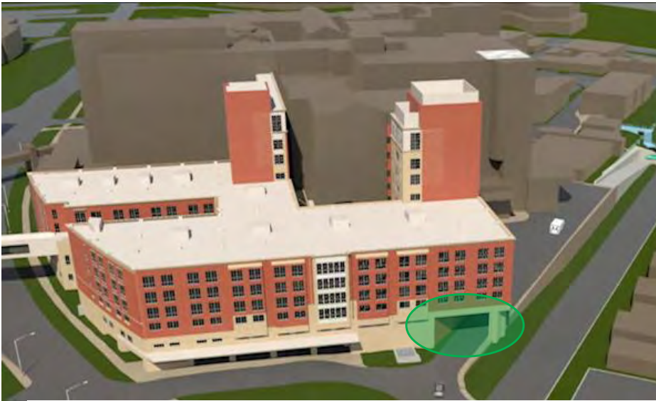
Figure 6 - Span over Emergency Access Ramp and Street Labels Image courtesy of Gilbane Construction
