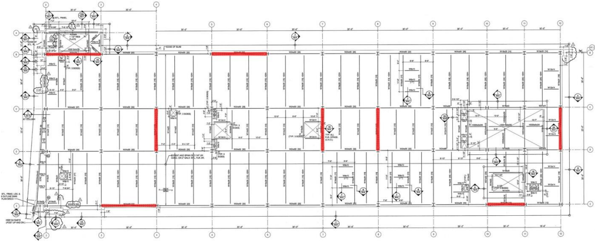
Figure 6 : Braced frame locations
