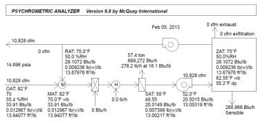
Figure 4: Central cooling coil sizing calculated with the McQuay Psychrometric Analyzer
