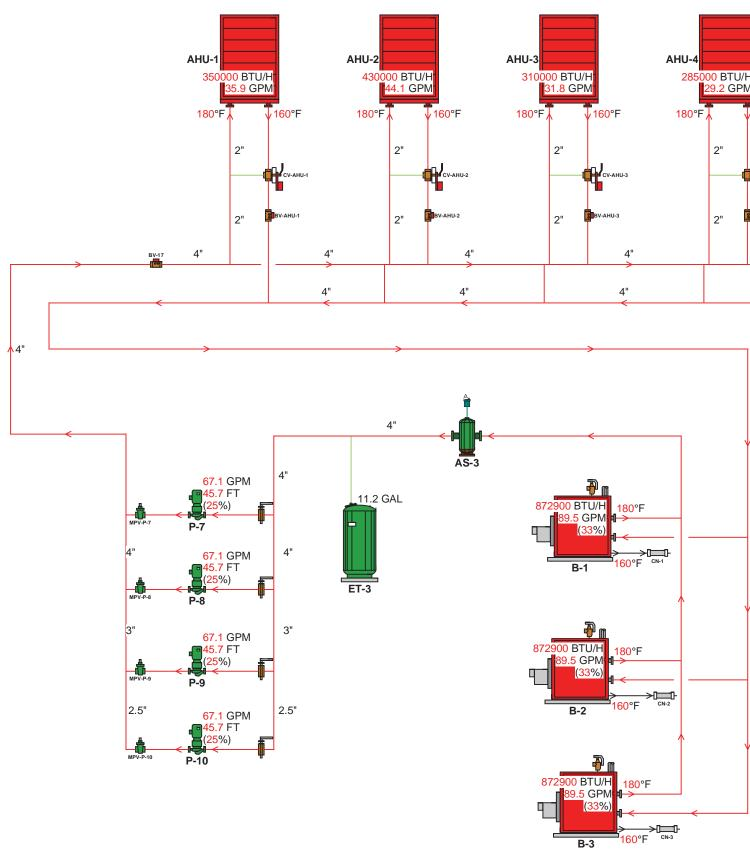
HEATING LOOP: Unlike the chilled water system, all heating loads could be placed on the same piping loop. All heated floor slabs are modeled as a single load at peak conditions. Supply temperature: 120F
