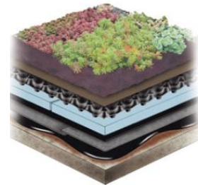
Figure 1: Ultimate Assembly for Plazas (American Hydrotech Inc., 2013)
