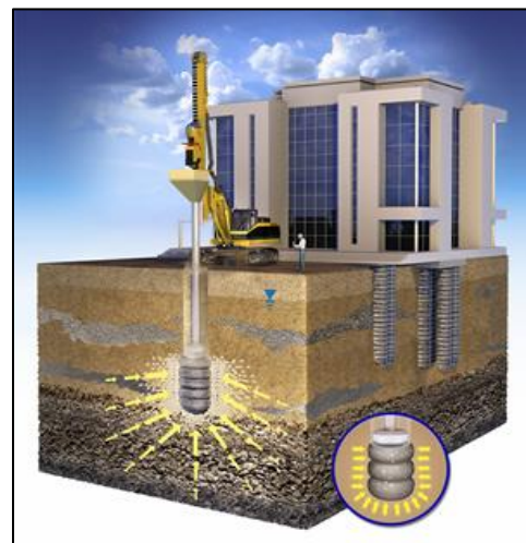
Figure 12: Rammed Aggregate Pier System 4
