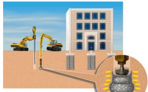
Figure 5 - Rammed aggregate pier construction (Image courtesy of www.buildinggreen.com )
