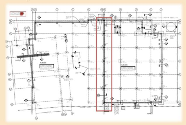
The original sequencing plan was to pour the wall, have the erection gang begin work of the first floor framing, and have the plumber come in and do his underground work around the steel team, then secure the foundation wall. There is a large amount of underground plumbing and mechanical work that needs to be completed next to the wall which can be seen in the drawings. The wall is not a retaining wall, and backfill could not occur until after all work was completed.
