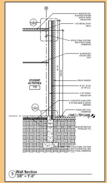
The geotechnical report found water in one of 26 of the holes that were drilled. Also, the spring that was located in both 2008 and 2010 was decided to be irrelevant to the foundation design. Because the Excavation is not excessively deep, the shallow footings were sufficient and no dewatering system or excavation support was needed.
