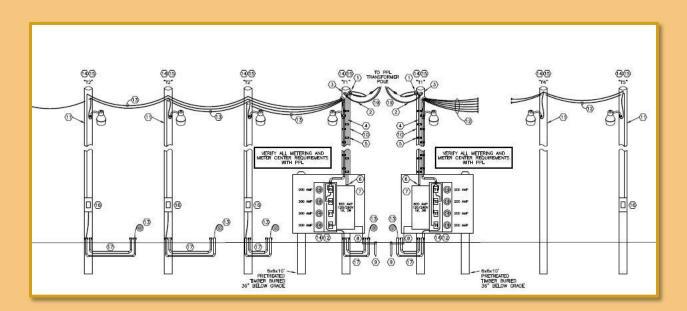
The permanent electrical system will be made to run the Student Life Building and Central Plant. There are two transformers feeding the building. Both will bring 12.5kV into the electrical room and step that down to 480/277 3 phase power. There is also an emergency generator that will supply power to the building and central plant if needed.
