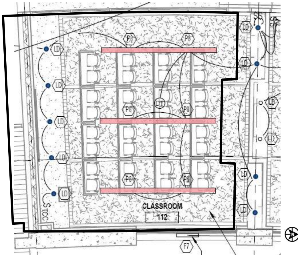
Figure 1.3 | Classroom Reflected Ceiling Plan
