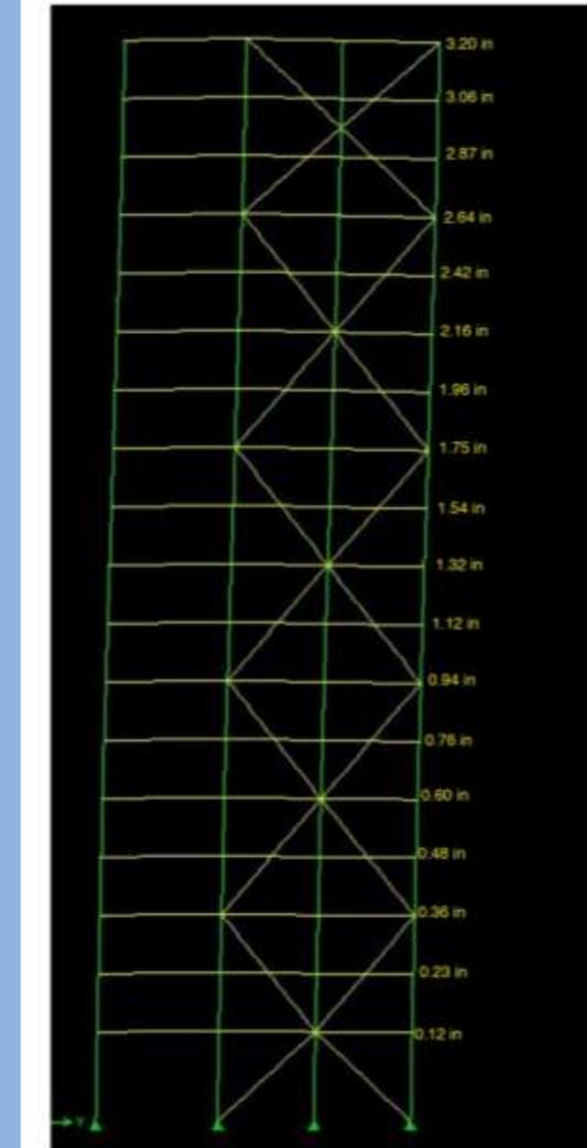
Deflections due to critical seismic loadcase in North-South direction (Not including P-delta analysis)
