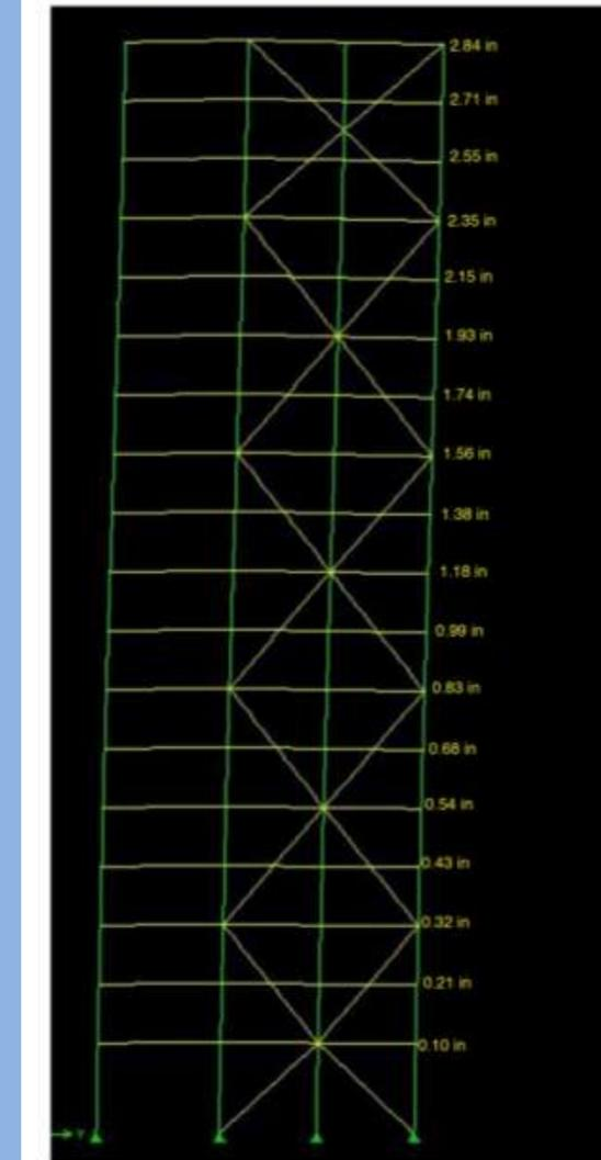
Deflections due to critical seismic load case in North-South direction (including P-delta analysis)
