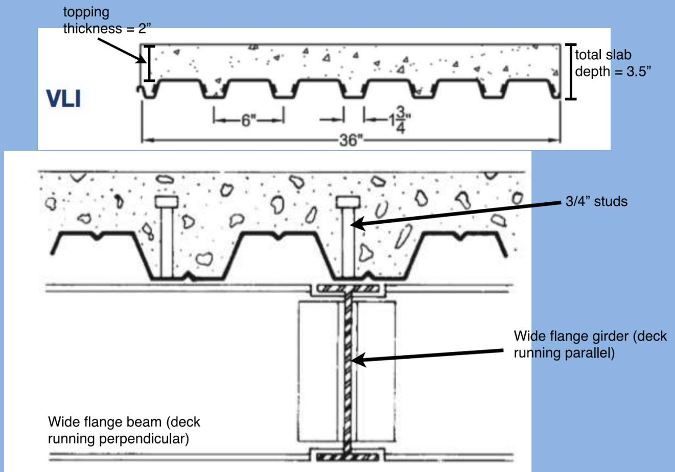
Typical cross-section of composite floor system
