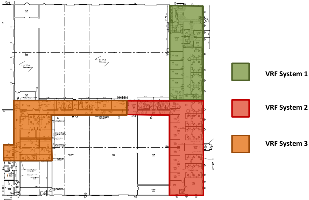
Figure 10: VRF System Area Layout
