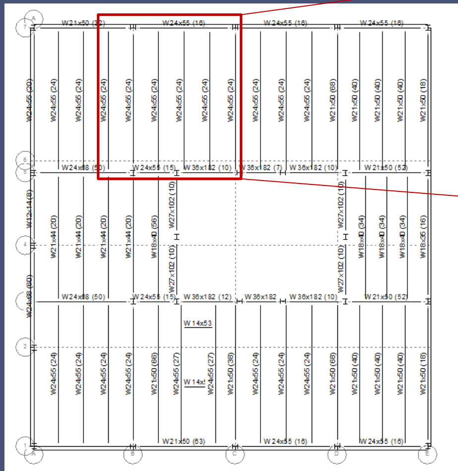
Typical Floor Beam Layout
