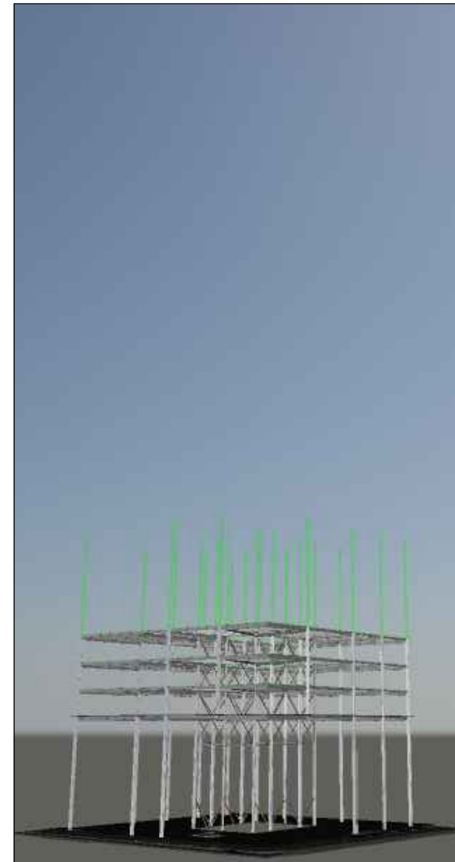
September 23, 2013: Structural steel associated with floors 5-8 are set in place. Floors 5-8 compose the first phase of repeated construction activity. As steel rises above to floors 9-12, floor decking and facade work will commence on the lower levels.
