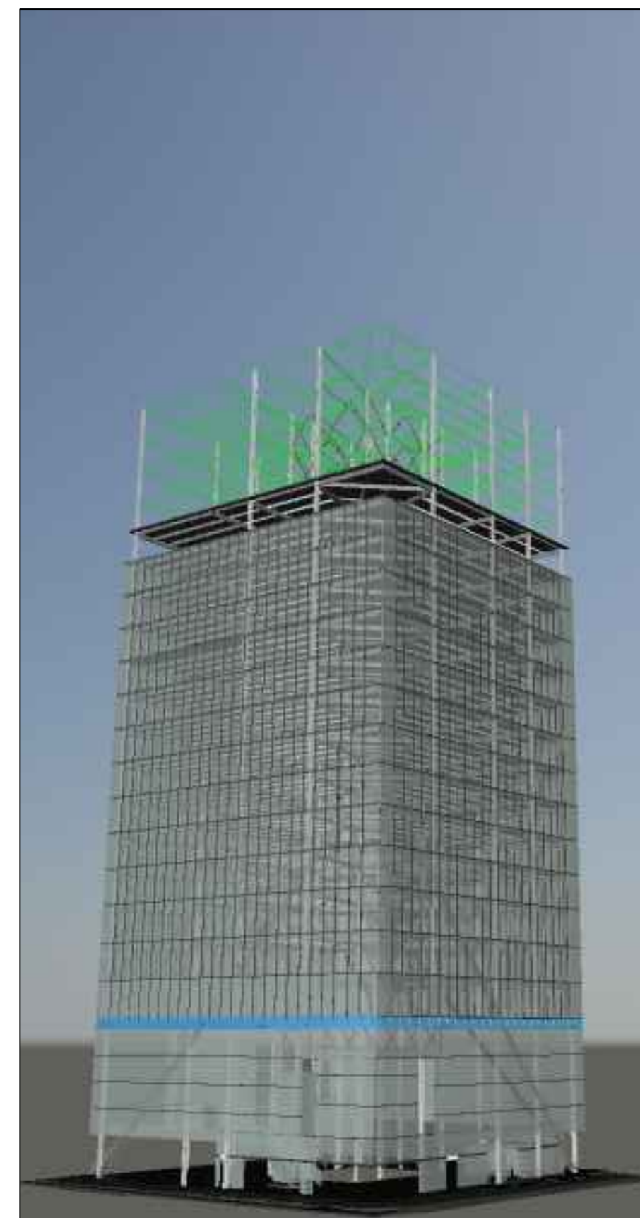
February 27, 2014: Structural beams and girders are installed on floors 17-20. Preparation continues on the installation of upper lateral beams. MEP installation now occurs on floors 9-12.
