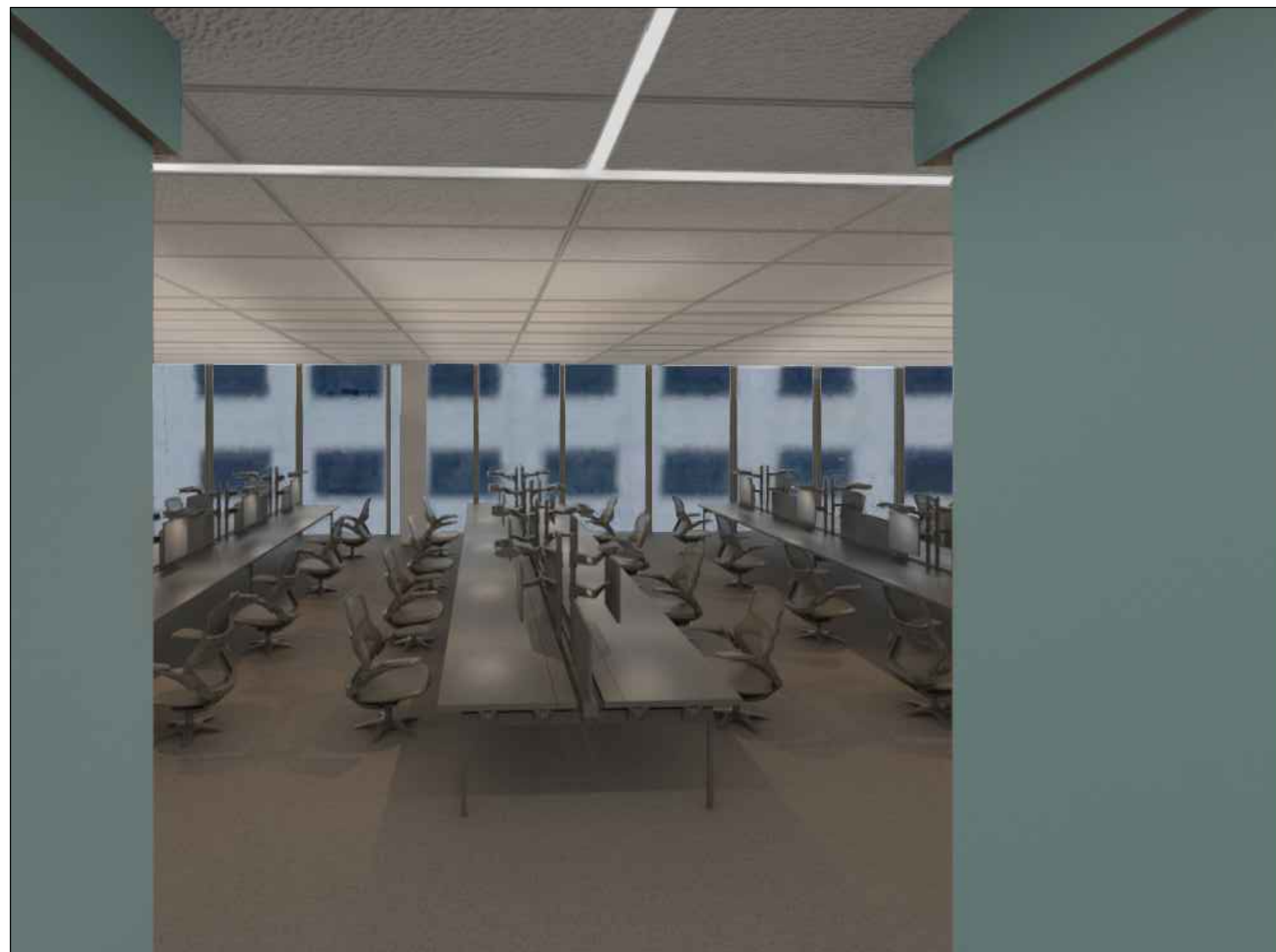
Left: Typical floor open office area. View taken from adjacent corridor. Furniture mounted lighting fixtures allow space for radiant panel layout.
