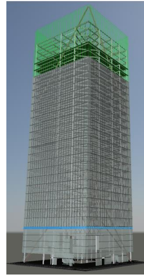
April 19, 2014: Structural columns and core reaches floors 21-24. Beams and girders will be set in place in the coming months. MEP installation commences on floors 13-16.
