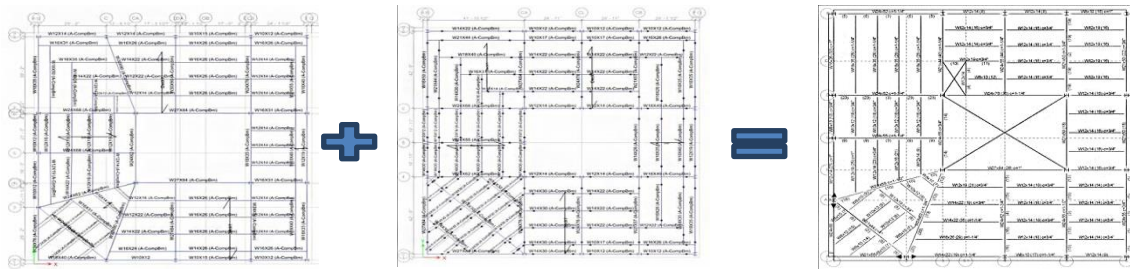
Figure 6: Two Potential Floor Beam Layouts and Finalized Layout (l-r: Angular, Revised Column, Final)
