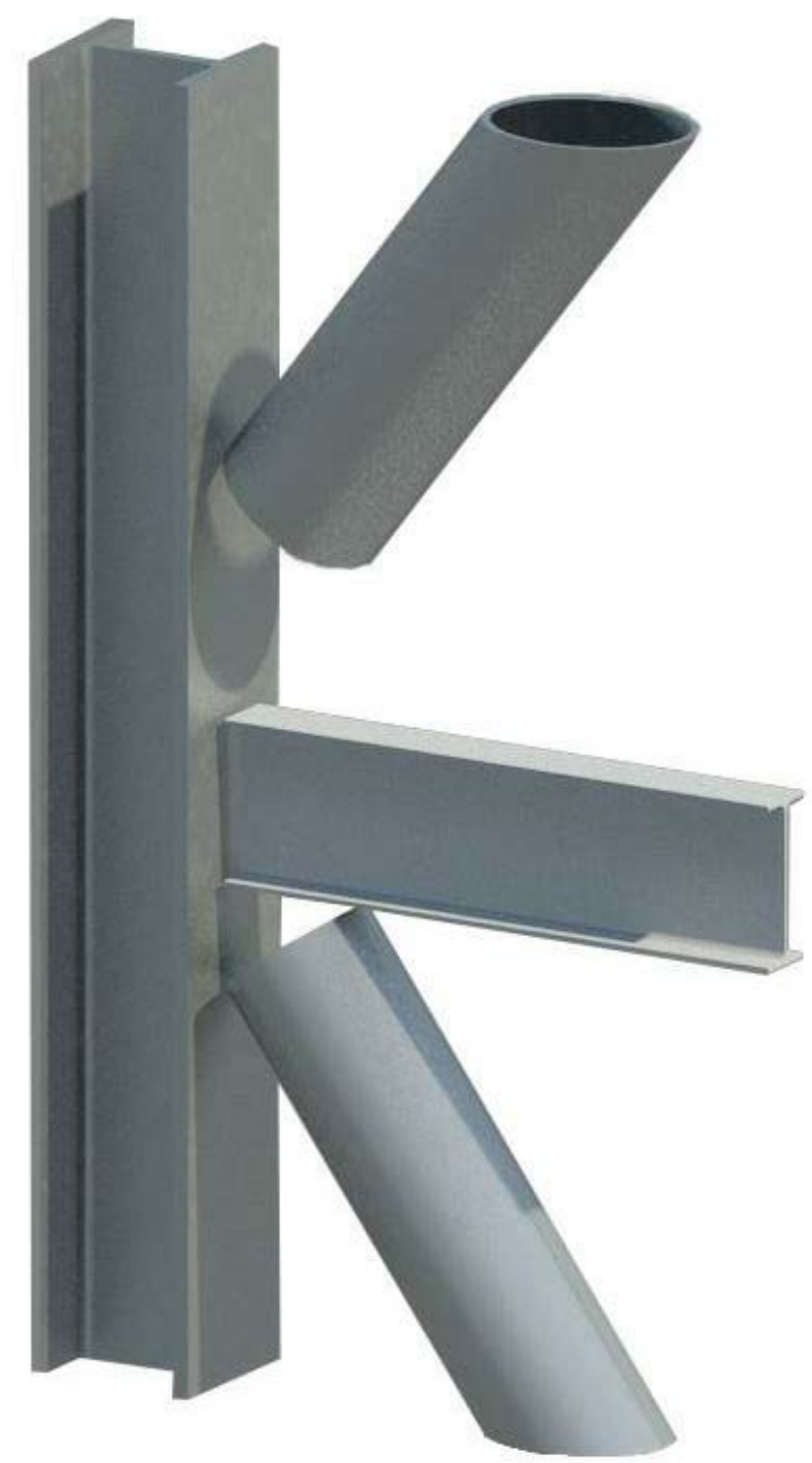
5 3D LATERAL GUSSET CONNECTION LOCATION RENDER N.T.S.
