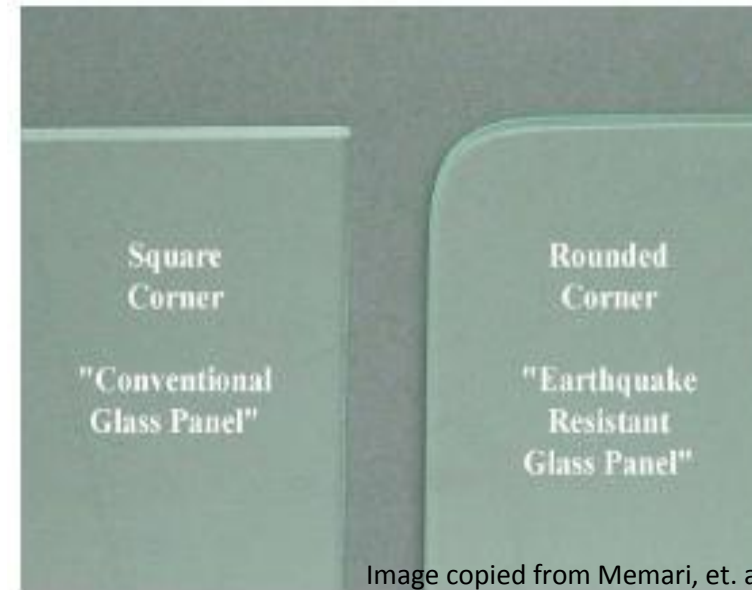
Image copied from Memari, et. al. Figure H.4: Schematic of Rounded Corner Glass (Provided by Memari, 2006)
