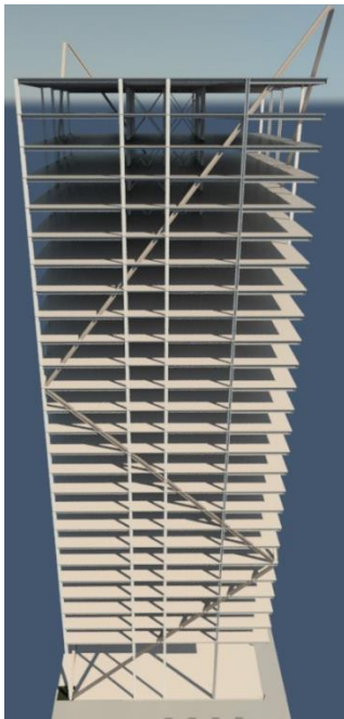
Figure 13: Exterior Bracing Elevations and
