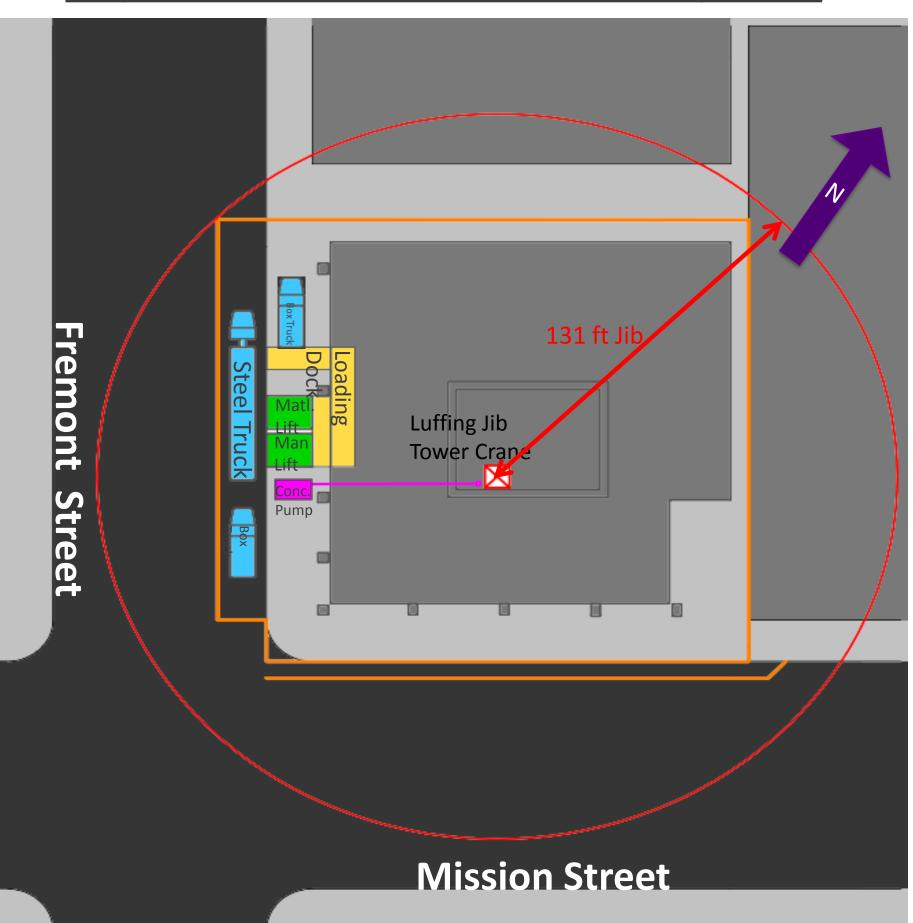
Once the building structure starts rising a material and man hoist will be needed to provide vertical transportation for both the workers and any material that will not be hoisted by the crane. To unload this material a loading dock shown in the delivery plan above will be constructed so material can be off loaded with ease.
