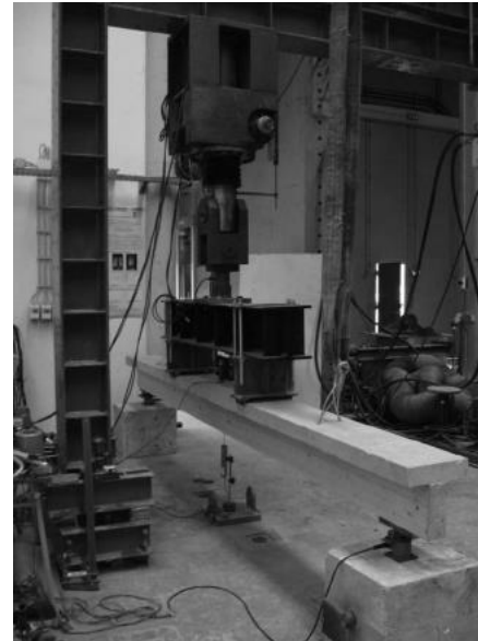
Figure 114: Bending test of glued composite member (Henrique et al.)
