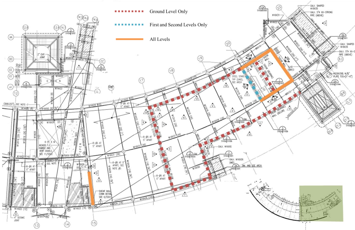
Figure 55: LFRS of east end of building
