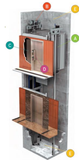
Figure 26. Machine-room-less elevator highlighting its (B) compact gearless machine, (C) compact controller, and (E) small hoistway
