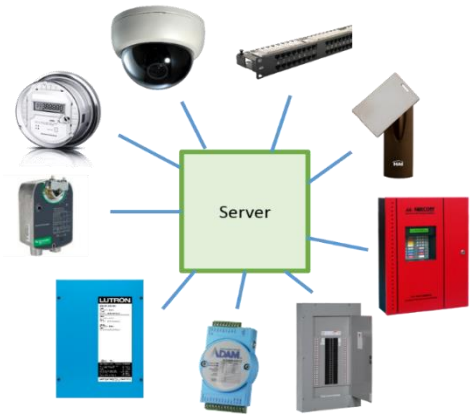
Figure 27. Building network system
