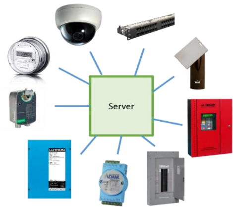
Figure 27. Building network system
