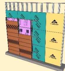
Figure 22. Rain screen façade
