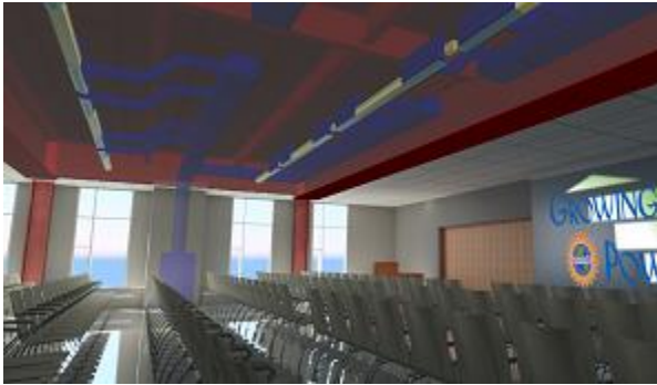
Figure 25. MEP linear scheme to coordinate with girders
