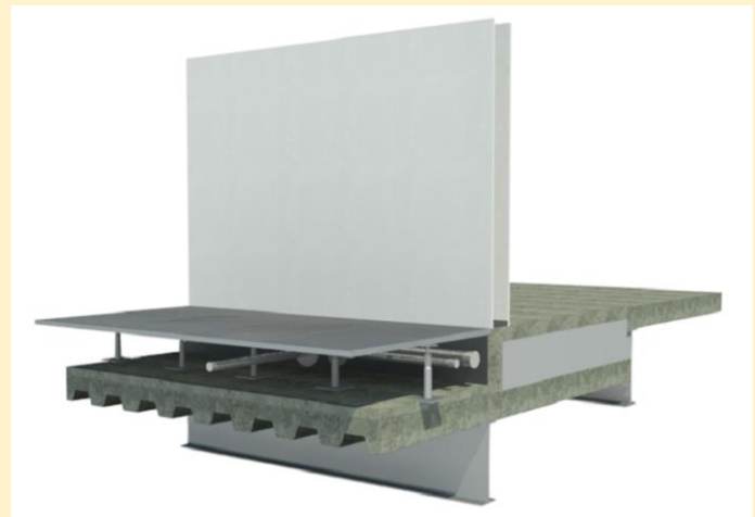
Figure 6. An elevated grate floor system in the greenhouse prevents piping from causing tripping hazards.
