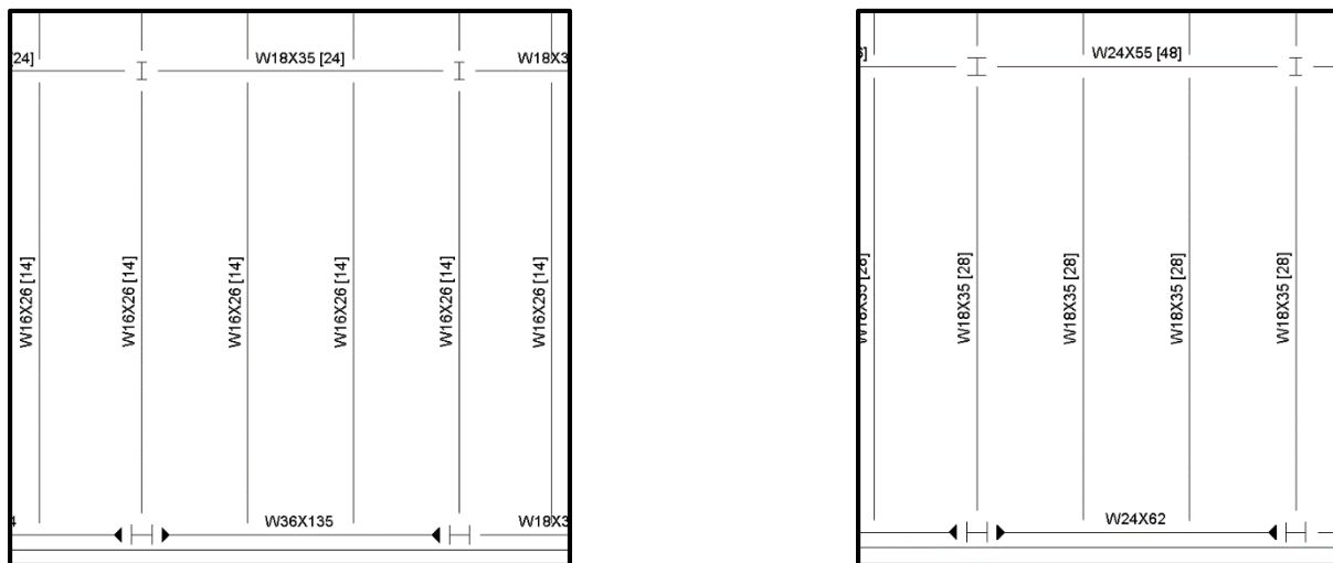
Figure 5. Typical steel bay supporting base building (left) and greenhouse (right).
