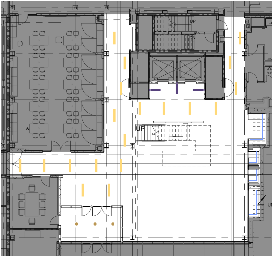
Figure 11 First Floor lobby and Corridor Lighting Plan
