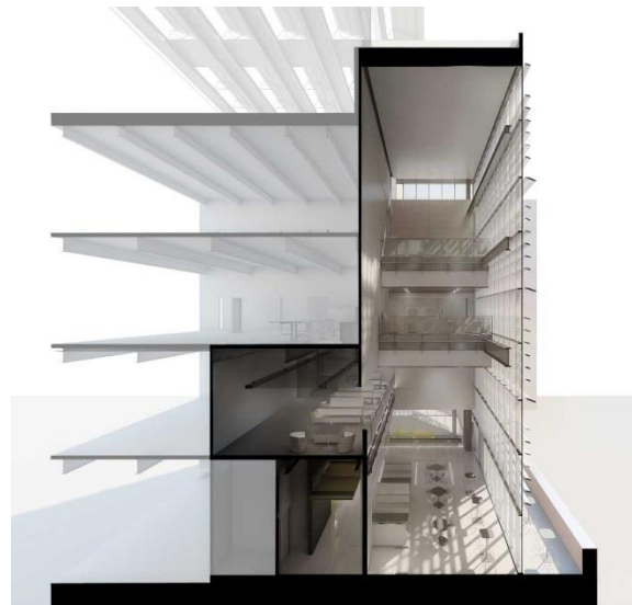
Atrium Section showing exterior glazing and shading louvers | Courtesy of SmithGroupJJR
