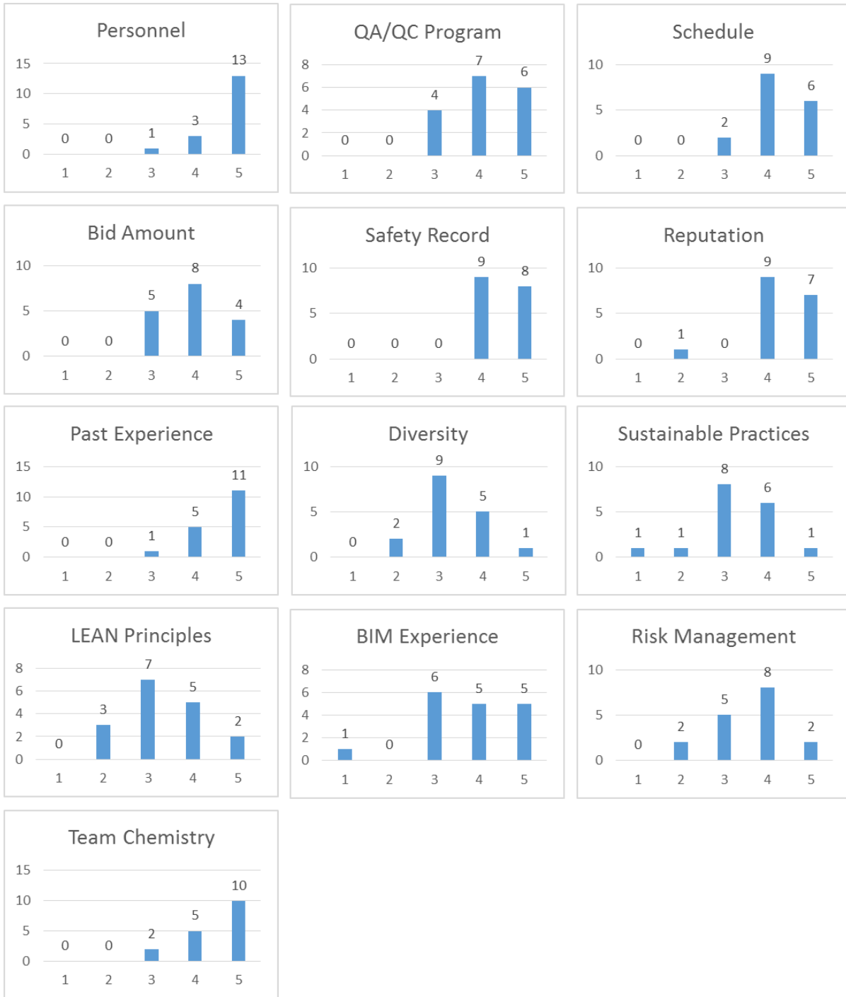
Figure 4-3: Returned values for the thirteen criteria when applied to MEP Subcontractor Selection
