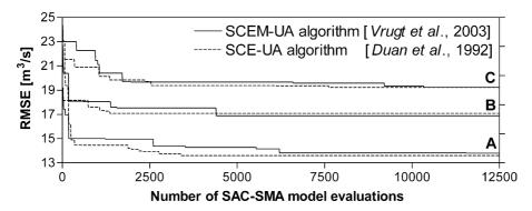
Fig. 9. Evolution of the 'best' parameter set, measured in terms of RMSE of the non-transformed flow for the SCE-UA and SCEM-UA algorithms using 2 (A), 5 (B) and 10 (C) years of calibration data.
