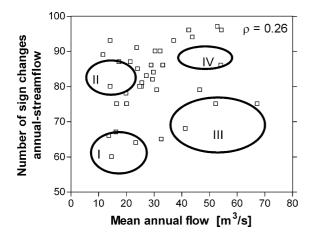
Fig. 8. Two-dimensional bi-criterion plot of the mean annual flow versus the number of sign changes of the measured annual streamflow for each of the 36 years of the historical record. The four different clusters are indicated with a circle.
