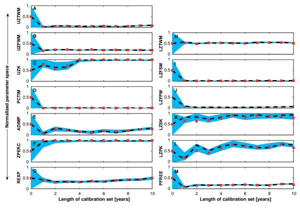
Fig. 1. Evolution of the 95% confidence intervals of the SAC-SMA model parameters as function of the length of the calibration set of measured streamflows in years. The evolution of the most likely parameter values is indicated with the solid line, whereas the SCE-UA solutions are indicated with the squared symbols.
