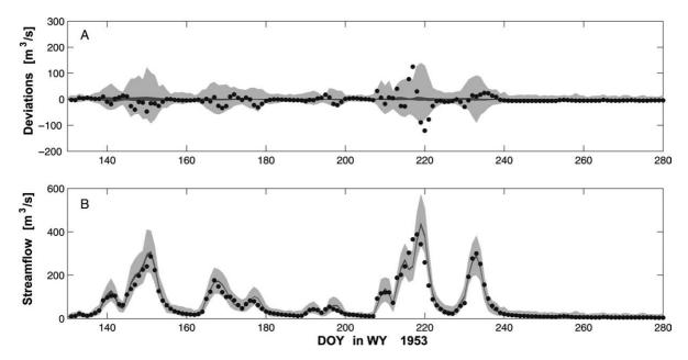
Fig. 4. (A) Streamflow uncertainties associated with the most probable parameter set derived using the SCEM-UA algorithm. The light-gray region denotes model uncertainty, whereas parameter uncertainty is indicated with the dark-gray region. The dots correspond to the observed streamflow data; (B) hydrograph prediction uncertainty associated with the uncertainty in the model (light-gray) and parameter estimates (dark-gray region) for the WY 1953.
