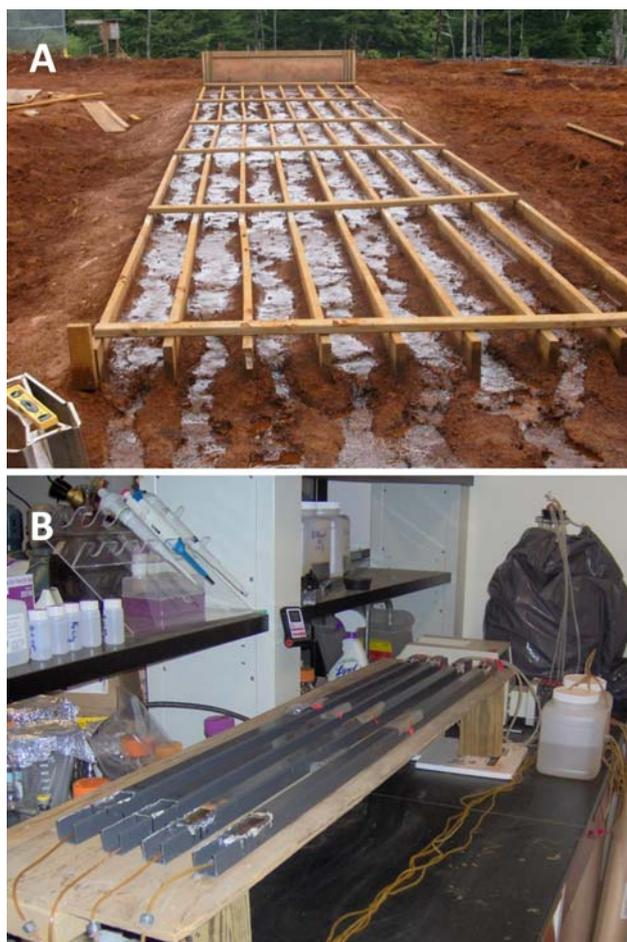
**Fig. 2** **a** Photo of the channel reactors built on the Hughes Borehole iron mound. **b** Picture of laboratory-scale gutter reactors showing the feed tank in the background and the four open-channel, flow-through reactors in the foreground
