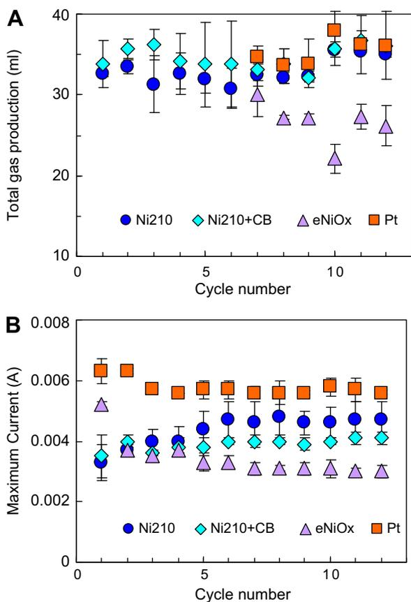
**Fig. 2 – (A) Total gas production and (B) maximum current for MECs with Ni 210, Ni 210 + CB, eNiO<sub>x</sub> or Pt catalyst cathodes, as a function of cycle number at an applied voltage of 0.6 V. Gas production for cycles 1–6 were not recorded for Pt and eNiO<sub>x</sub> due to equipment malfunction.**
