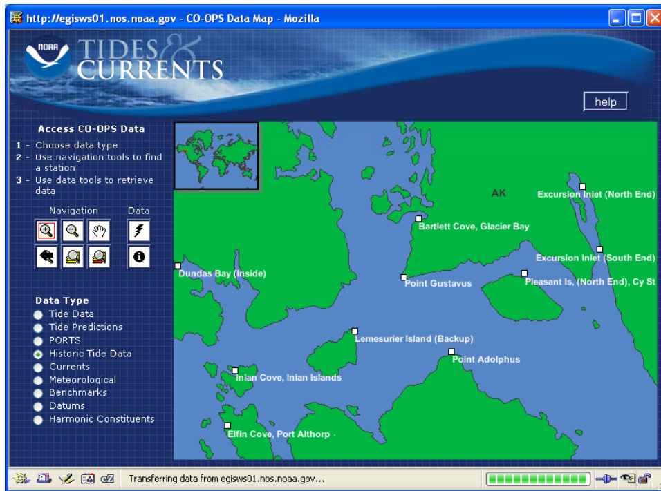
Figure 8.2: Interactive map allowing for the extraction of historic tidal data and tidal predictions.
