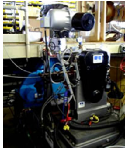
Figure 1: Ricardo “Hydra” Single-Cylinder Spark Ignition Engine used in the studies of hydrogen enriched natural gas combustion
