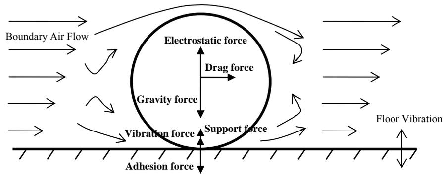
**Figure 1.** Force analysis on surface residing particles
