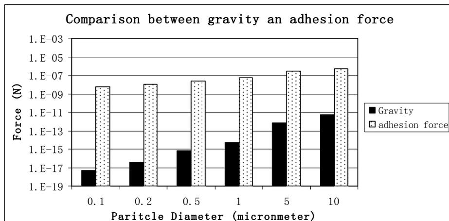
**Figure 2.** Comparison between adhesion force and gravity force
