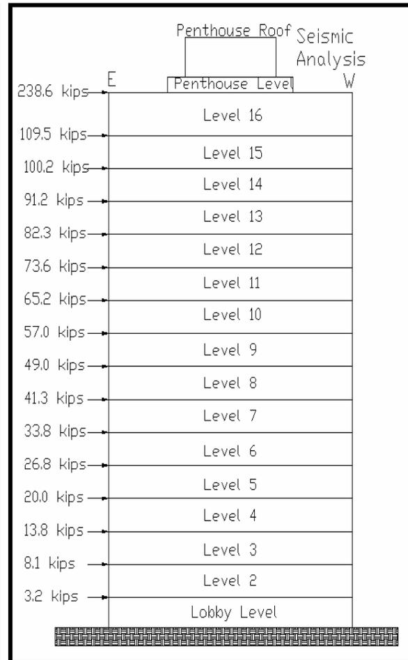
Figure 1.5-Seismic loads resolved to floors (E-W)
