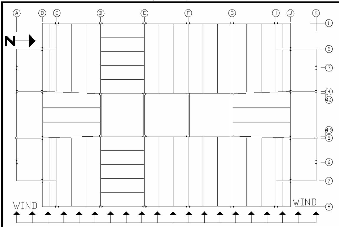
Figure 1.4- Wind force on E-W side of structure
