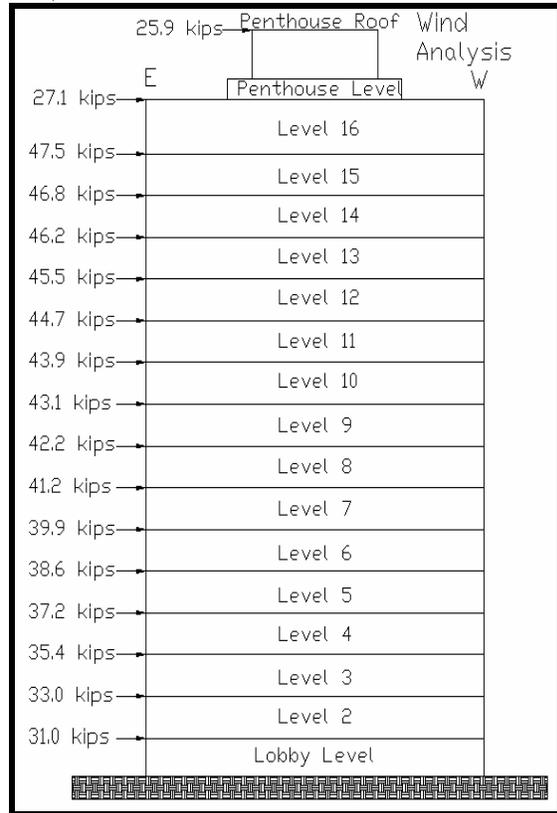
Figure 1.3- Wind loads resolved to floors (E-W)
