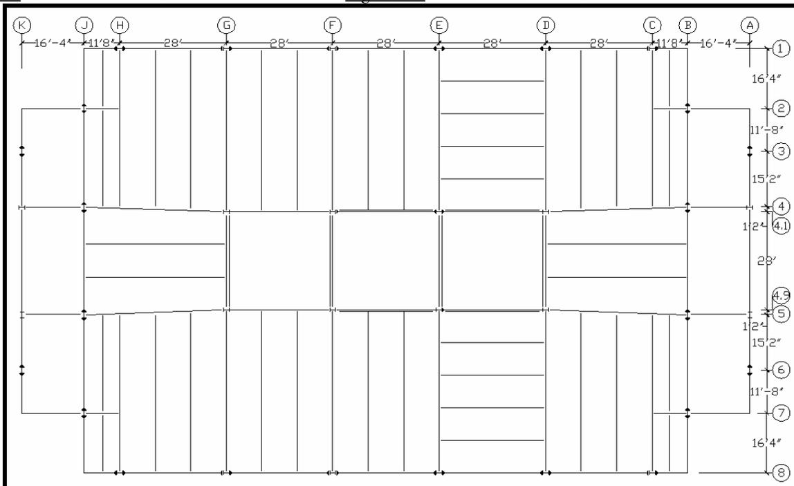
Figure B.3- Typical Framing Plan (Floors 3-15)
