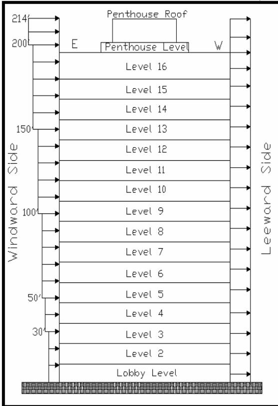
Figure 1.2- Vertical profile of wind loads
