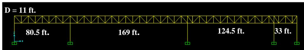
Figure 37: Planar Truss Model (Design 1)
