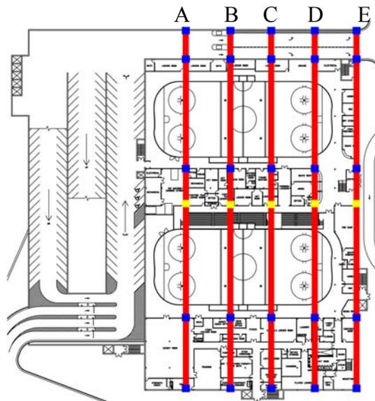
Figure 39: Design 2 Truss and Column Locations
