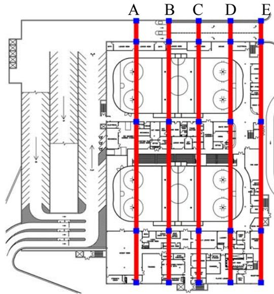
Figure 36: Design 1 Truss and Column Locations
