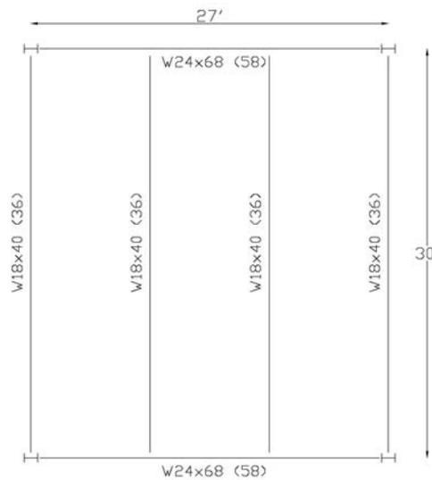
**Figure 7: Enlarged Typical Framing Plan**
