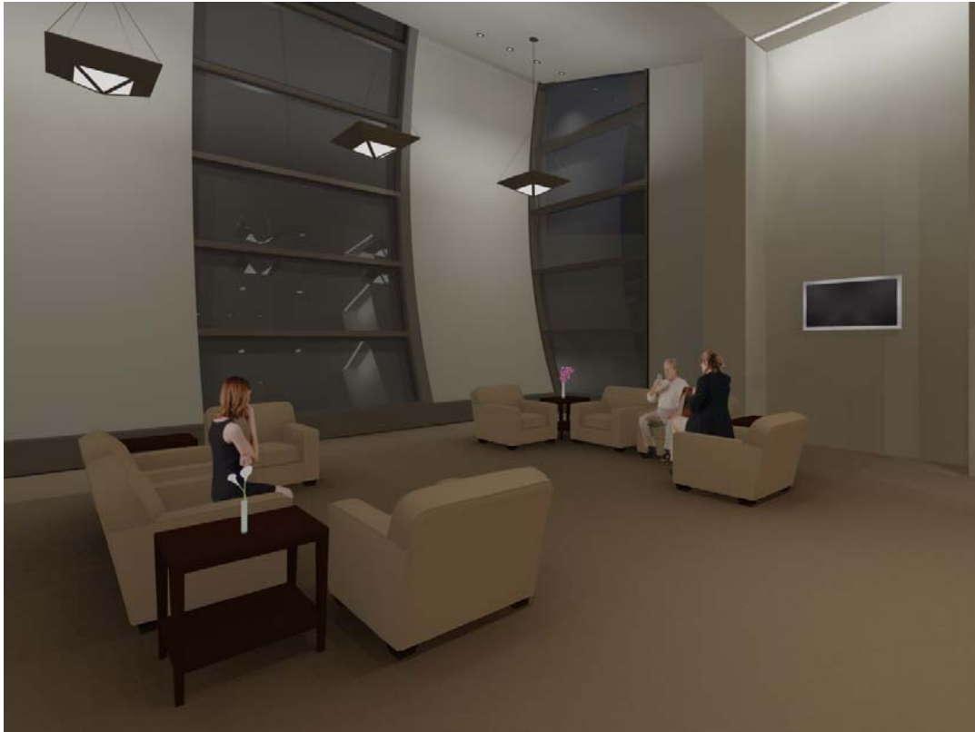
Figure 4.4.3 | Meeting room view with pendants (30%) and downlights (10%) dimmed to create a more relaxed environment.
