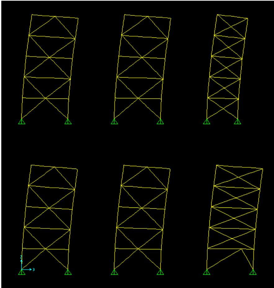
**Figure 23:** Deflected Shape of Braced Frames in Sap 2000
