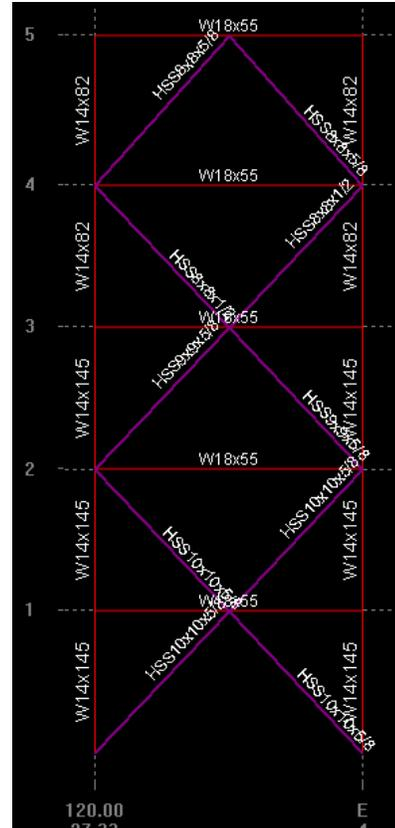
Figure 17: Braced Frame 2
