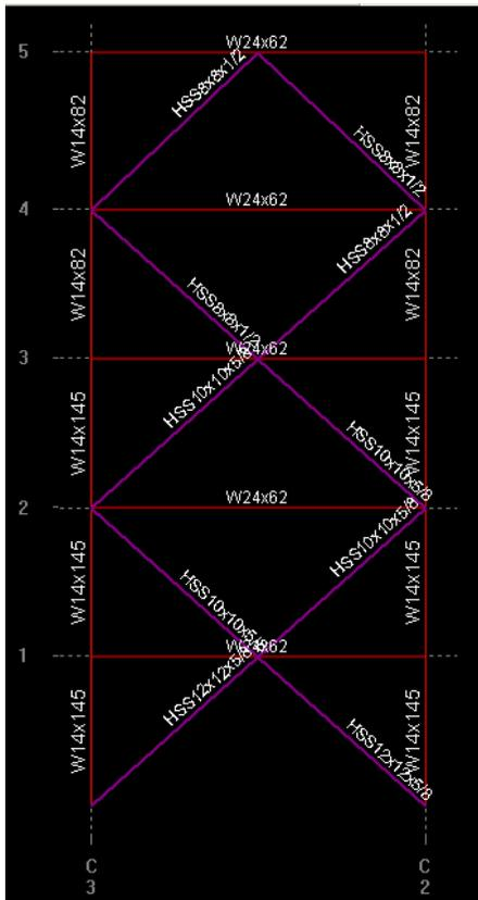
Figure 16: Braced Frame 1
