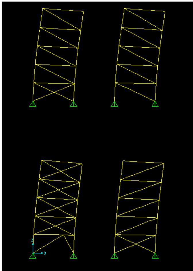
**Figure 13:** Deflected Shape of Braced Frames in SAP 2000
