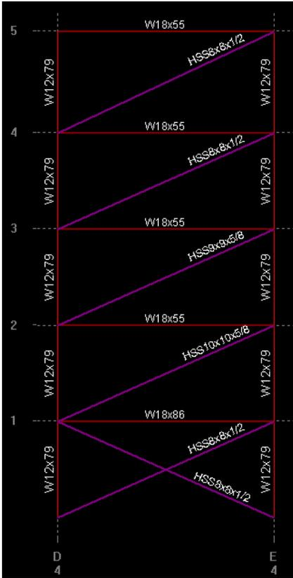
**Figure 10:** Braced Frame 2
