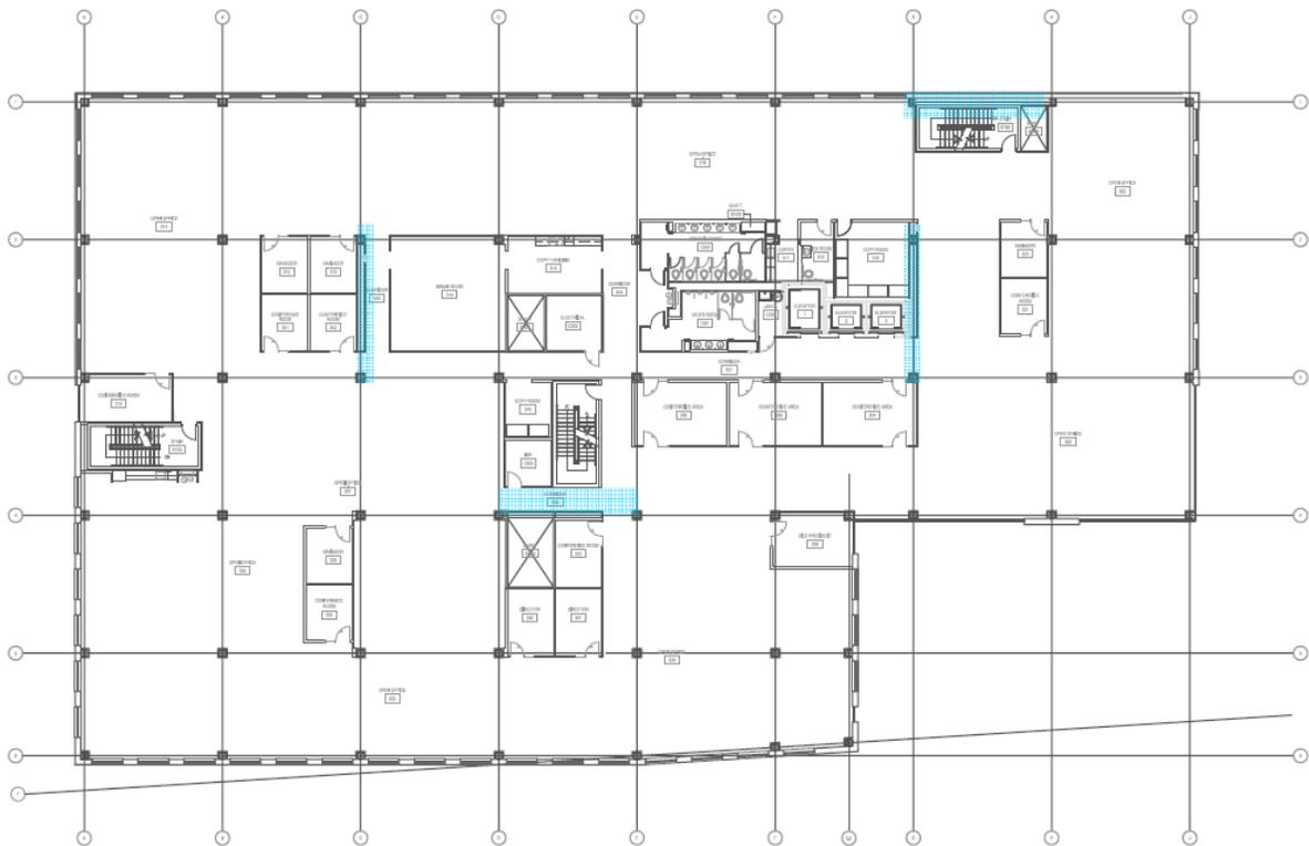
**Figure 29:** Remaining Original Floor Plans and Location of Braced Frames
