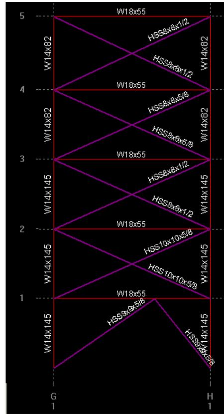
**Figure 21:** Braced Frame 6
