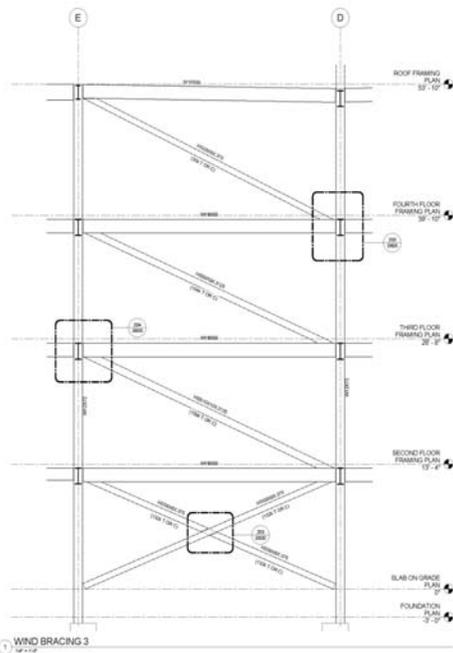
**Figure 4: Braced Frame 1 Elevation**
