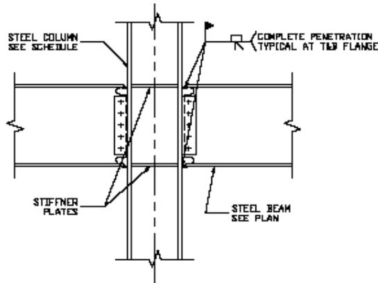
**FIGURE 1** – Typical Beam to Column Moment connection
