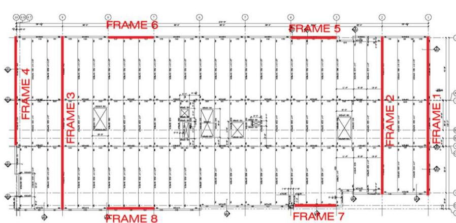
**FIGURE 2** – Typical Floor plan with moment frames
