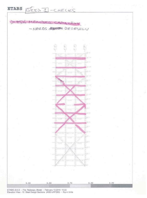
Additional hand calculated checks (Grid I) were performed to provide validity of the ETABS analysis.
