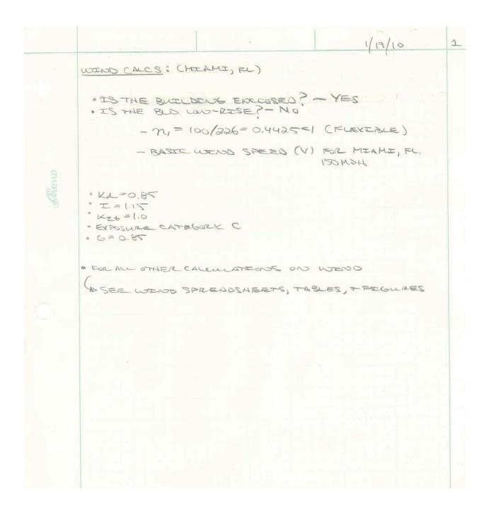
The following tables provide excel spreadsheet calculations for determining the wind forces acting upon the building in Miami, FL. These calculations conclude with story forces, story shear, and overturning moment values.
