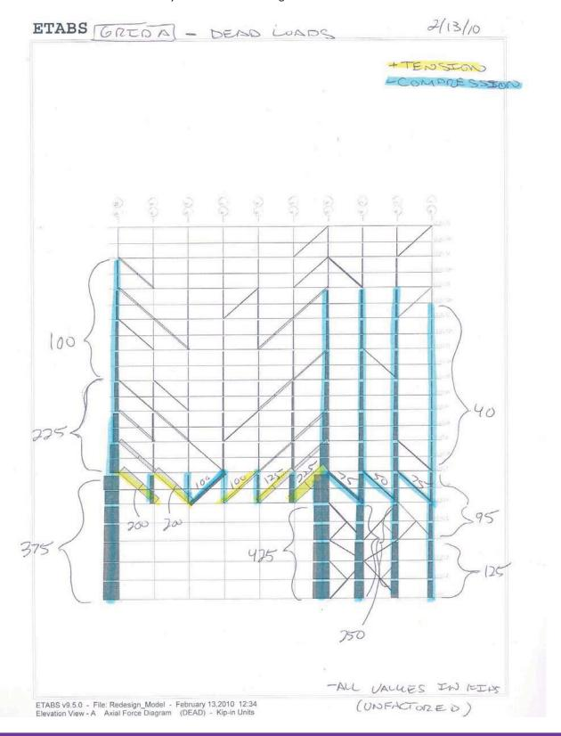
Below is example hand calculation checks performed for Grid A.
