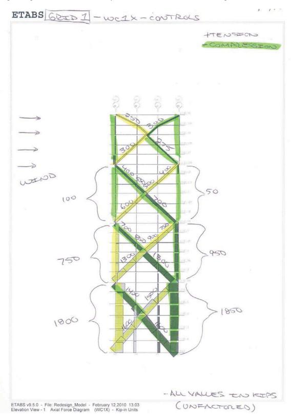
Below is a preliminary design of Grid I bracing members. The members were treated as concentric (axial loaded) members. Member sizes were chosen appropriately using the LRFD (Load & Resistance Factor Design) manual.
