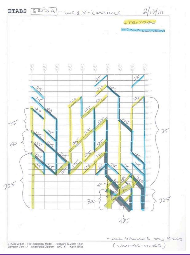
Below is an ETABS printout of mainly compressive forces in Grid A. Grid A is in the North-South direction of the lateral system. Grids A, C, & D have lateral members that are loaded under both wind and dead load forces. Combinations of these forces are analyzed to check the design of column and brace frame members.
