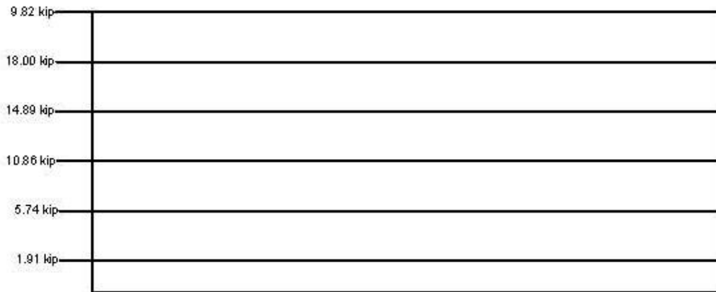
Figure 11.b: E-W Wind Load Story Shear.
