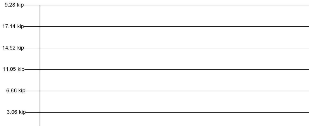
Figure 12.B: N-S Wind load story shear.
