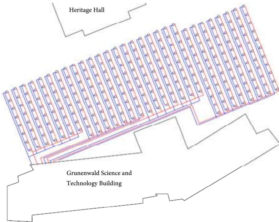
Figure 13- Proposed Geothermal Borehole Layout
