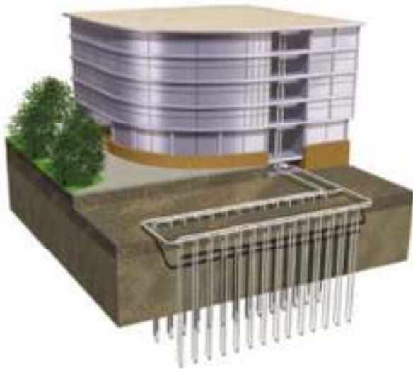
Figure 7- Vertical Piping Layout
