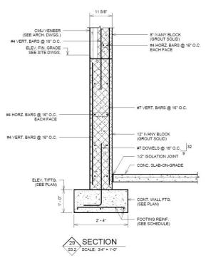
Figure 2: Typical Ivany Block Wall
