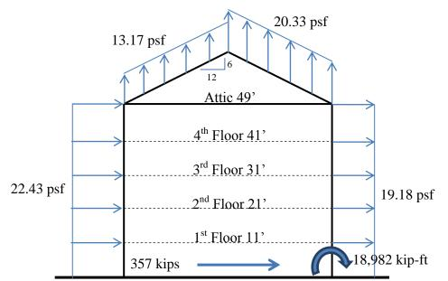
Figure 5: E-W maximum wind pressures for the hip roofs of the wings The shear and moment are for the entire structure.
