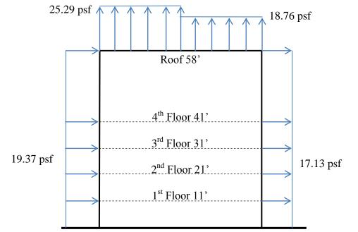
Figure 6: N-S and E-W max wind pressures for the flat roof of the central core
