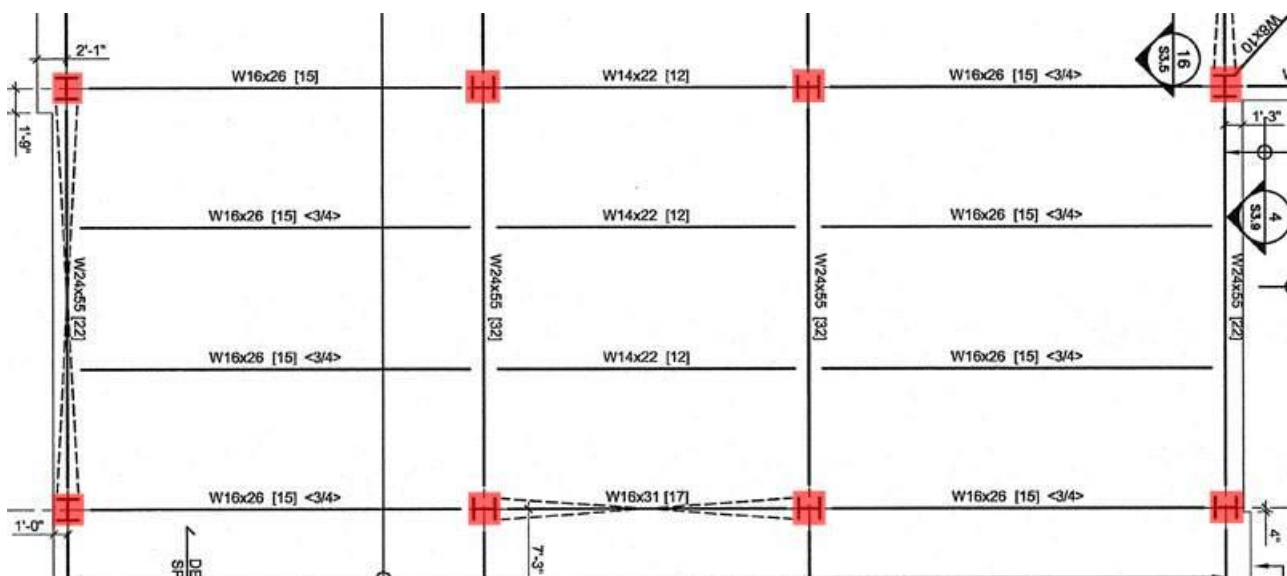
Figure 5: Typical column layout
