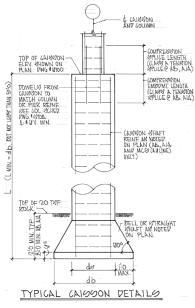
Figure 1. Typical Caisson Detail
