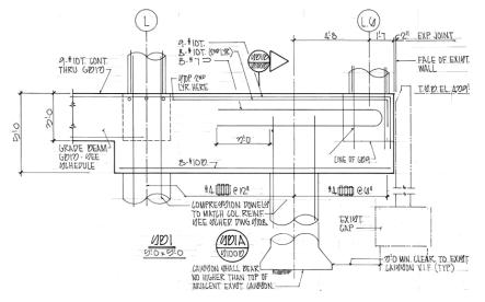
Figure 2. Example of caisson and column misalignment
