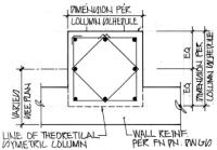
Figure 10. Illustration of Column Used for Support of Architectural Cylinder
