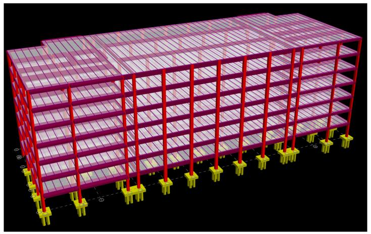
Figure 12. Model of BMR viewed from the south face. It should be noted that the north and east sides of the building have additional buildings that would impact the amount of wind that this building would see. The south and west sides are exposed.
