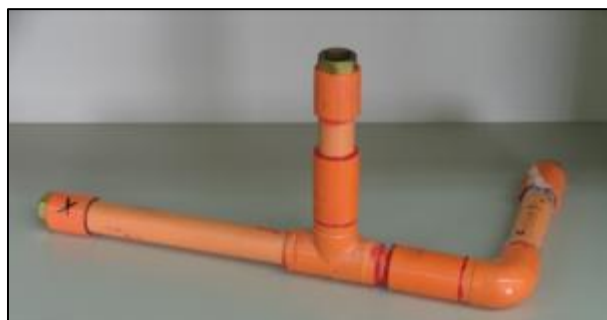
Figure 4 CPVC Sprinkler System Image from www.exponent.com
