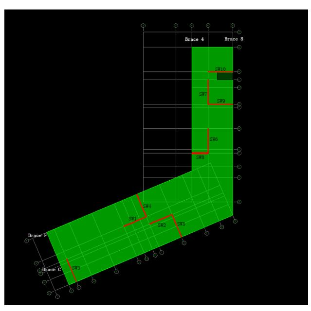
Figure 10: Shear wall locations of a typical floor
