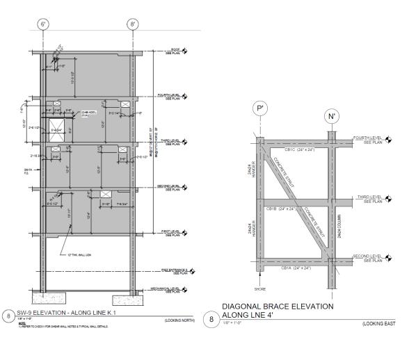
FIGURE 8: TYPICAL CONCRETE SHEAR WALL
