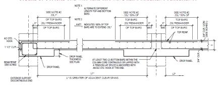
FIGURE 6: TYPICAL COLUMN STRIP DETAIL WITH DROP PANEL AND EDGE BEAM
