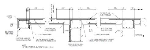
FIGURE 5: TYPICAL ONE WAY SLAB SHOWING REINFORCEMENT PLACEMENTS
