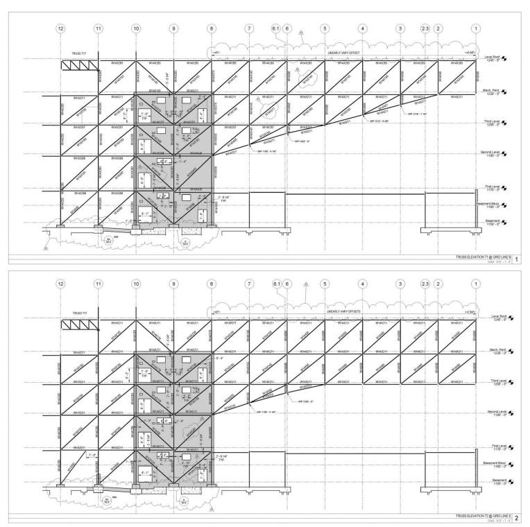
Figure 16: Truss frames at column lines 2 and 5; also replicated at column lines B and E.
