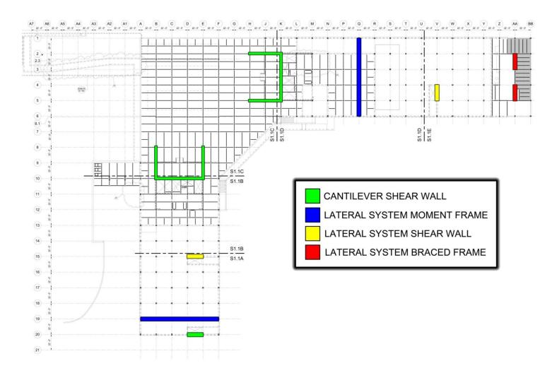
Figure 15: First floor lateral system elements
