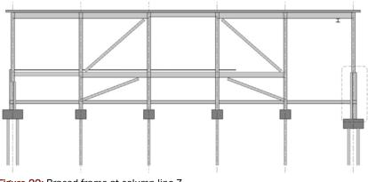
Figure 22: Braced frame at column line Z
