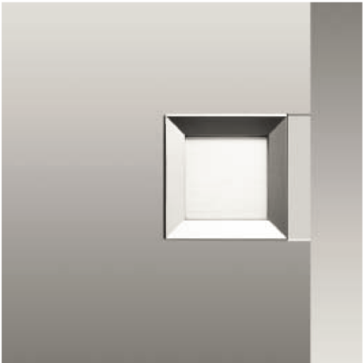
Wall or ceiling mounted luminaires with die cast aluminum frame/guard. Heavy pressed ¼" thick crystal glass with internal structure and white translucent ceramic coating. U.L. listed, suitable for wet locations. IP 65. Color: Standard BEGA finishes.
