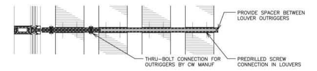
The image above is the plan view of the solar shade connection system.
