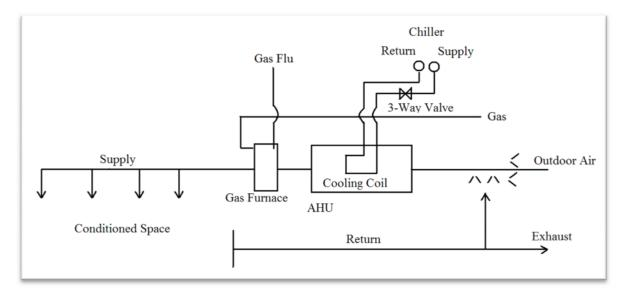
• Figure 20 – Schematic of Chiller Based Mechanical System
