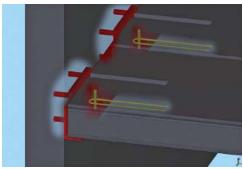
Figure 6: Principle connection of deck elements with interior concrete shear wall.
