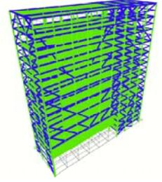
Wind Case Forces Calculated & Inputted into ETABS Software – Analyzed
